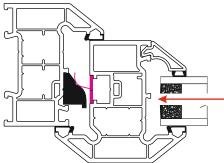
It may be necessary to pack the sash/glass at this point as shown
